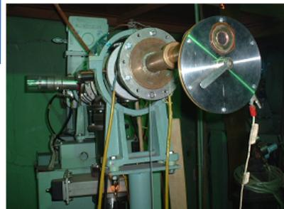
Low beam current irradiation chamber for RT irradiation
