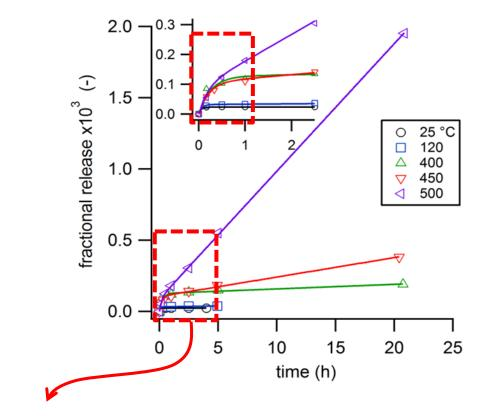
At low T, fraction of Po is released unexpectedly fast
