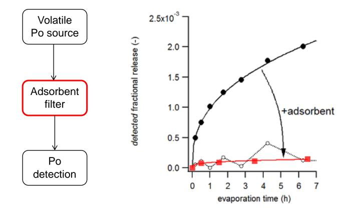
Activated carbon efficient adsorbent for volatile Po
