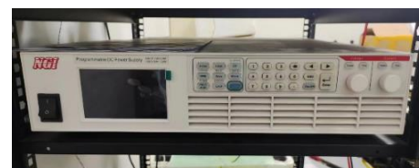
Power supply in the CLIQ system
