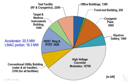
Figure 13: Power consumption breakdown of the spallation neutron source (SNS)
