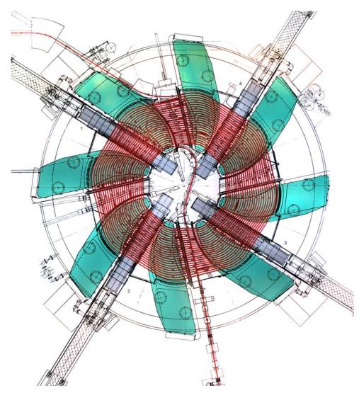
Figure 9: The 590MeV isochronous cyclotron at PSI with a diameter of 15m.
