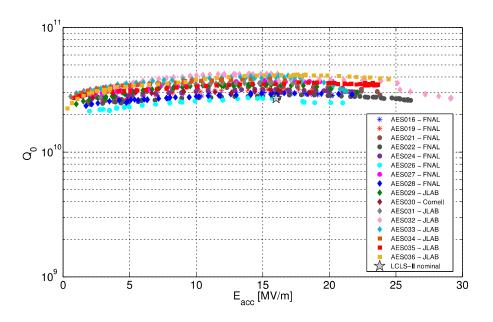
Figure 19. Q<sub>0</sub> versus the acceleration gradient for dressed LCLS II cavities (A. Grassellino).
