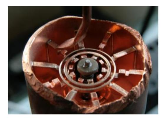
Figure 7: Cross section of a typical microwave cooker magnetron (Brian Chase, FNAL).
