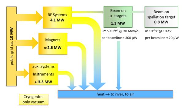
Figure 11: Breakdown of PSI HIPA facility power consumption.
