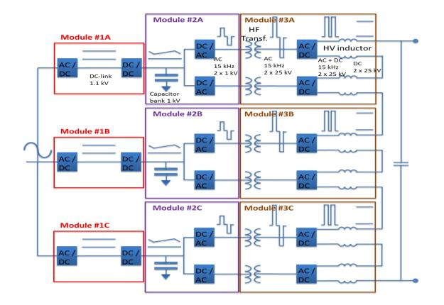
Figure 4: Topology of stacked HF transformer based modulator developed by ESS (Carlos Martins, ESS).
