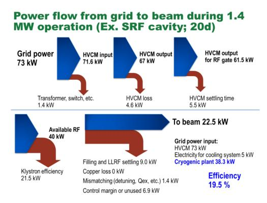
Figure 14: Example of power flow of a SRF cavity.
