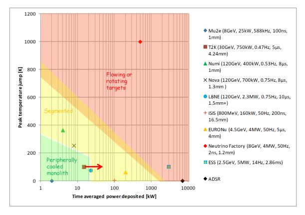
Figure 3: Time averaged power deposition vs. temperature jump.
