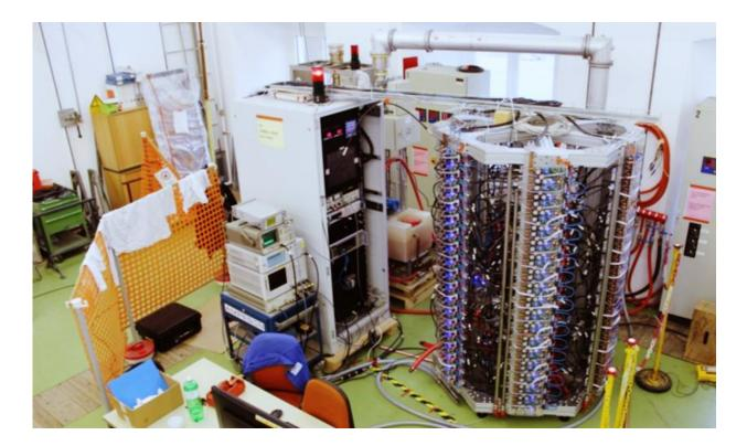
Figure 6: 65 kW, 500 MHz solid state amplifier at PSI (Marcos Gaspar, PSI).
