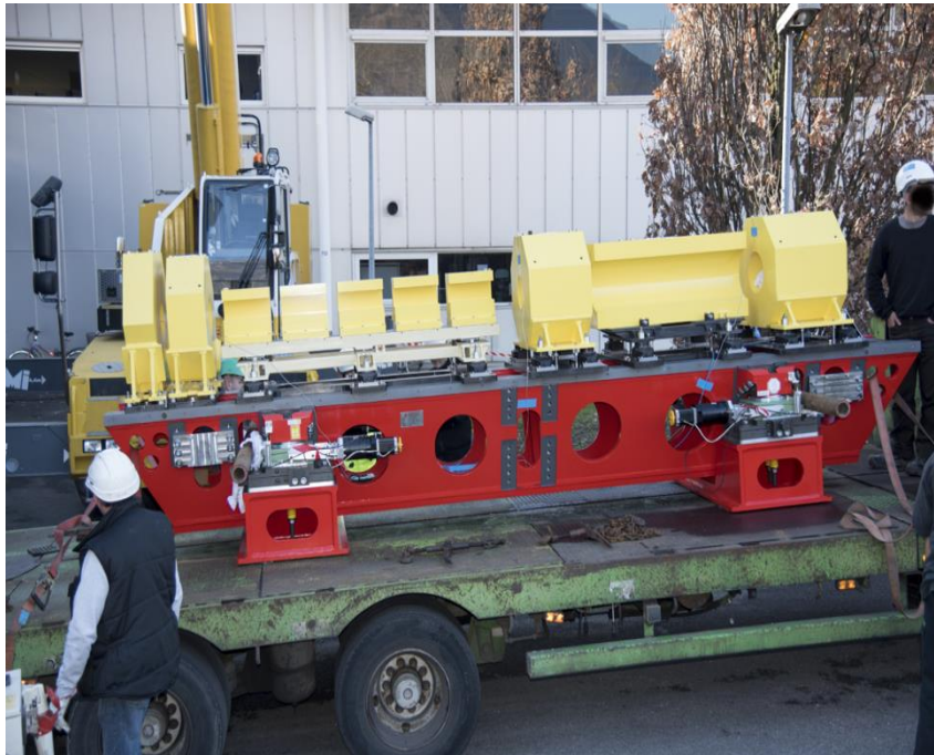
Girder prototype with dummy magnets: Mechanical tests
