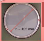
Foil 3 $\mu$ m MYLAR + 5 $\mu$ m CsI(Tl) CCD camera Hamamatsu Orca 4.0/IDS 54k ph/MeV,  $\lambda_{MAX}$  550nm =CCD Surface Muon 1200phs
