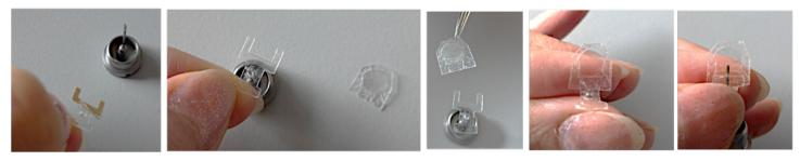
**Step 2.2.** Trim the corners of the well with a sharp scissors leaving a continuous strip of double stick tape around the edge of the well for structural stability. The trimmed well must be small enough to fit comfortably into a cryo-vial. Trim a minimum off one side of the well to expose the precipitant solution. By touching the precipitant with a cotton bud, gently wick away most of the precipitant from around the mesophase bolus.
