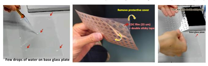
**Step 4.** Take the second COC film and remove the remaining protective cover from the film, place it with its non-silanized surface down and center it 2 mm from each edge on the cover glass plate to which has been applied a drop of water to bond the two by capillarity. With a clean tissue, force out excess water. This creates the cover plate with which to seal both the COC plate and the glass sandwich plate.
