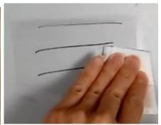
**Step 2.** Remove the protective cover from one side of the perforated double-stick spacer tape and apply it, sticky side down, to the silanized surface of one of the COC films from Step 1. Use the brayer to produce a tight seal. This step provides the COC base plate plus wells in which crystallization will take place.
