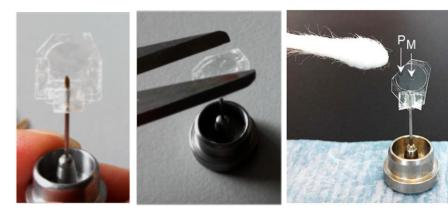
**Step 3.** Immediately plunge the well into a loading Dewar filled to the brim with liquid nitrogen. When the sample has equilibrated thermally transfer it into a precooled storage puck in the same loading Dewar. Using the mark on the bottom of the goniometer base orient the base in the puck to ensure the well will be aligned correctly in the beam and in the cryo-stream upon manual or robotic mounting. Place the puck in a shipping Dewar and ship to the synchrotron.
