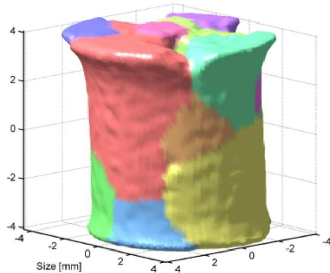
Grain mapping of polycrystalline bulky aluminum cylindrical sample.
