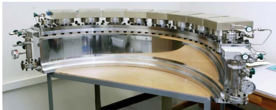
High-Efficiency 2D Detector for DMC and ERWIN
