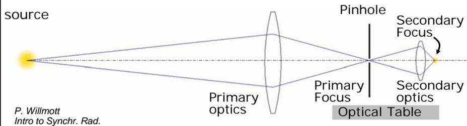
Typical undulator source size:  $200\ \mu\text{m} \times 20\ \mu\text{m}$
