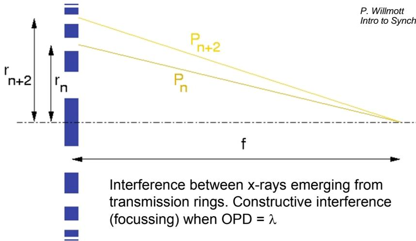
Interference between x-rays emerging from transmission rings. Constructive interference (focussing) when  $OPD = \lambda$
