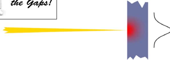
Scintillator plate plus e.g. 2D array of photosensitive elements such as a CCD array can be used to record x-ray images.
