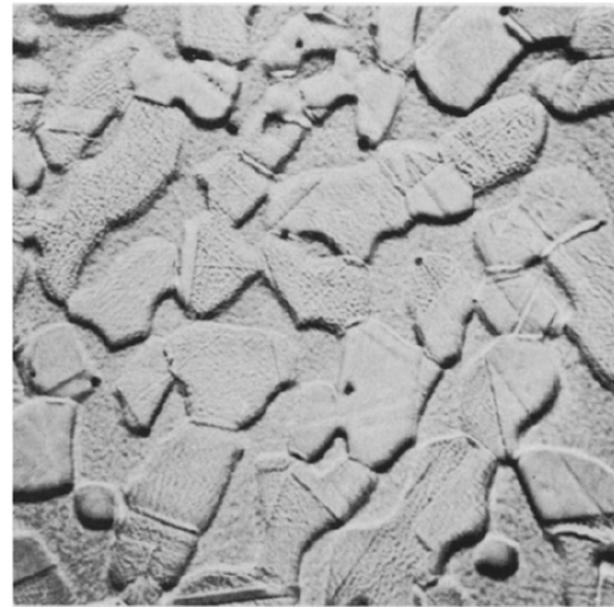
Ferrite grains swell less than austenite grains due to different swelling rate and different temperature regime of swelling
