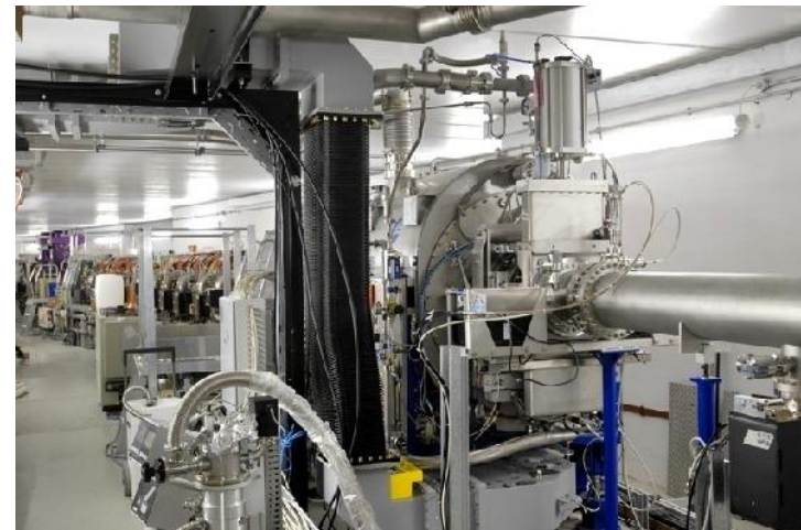
RF cavities to replace energy losses due to the emission of synchrotron radiation
