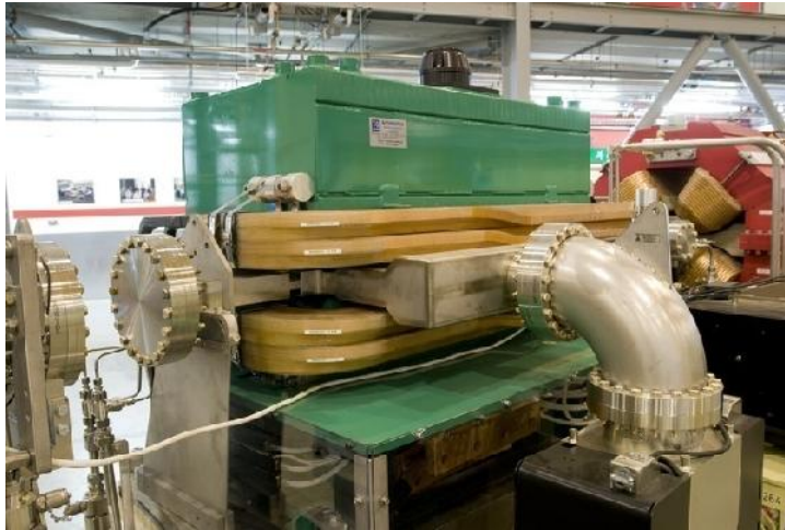
Sextupole magnets to focus off-energy electrons (mainly)
