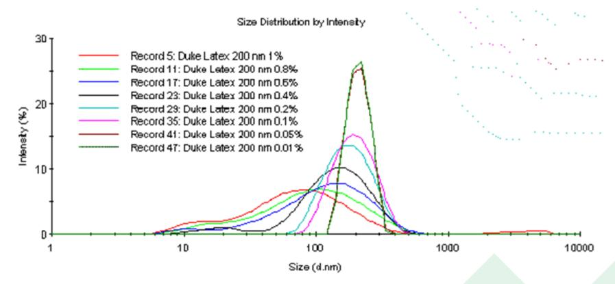
Latex 200nm measured without NIBS <u>in the center of a</u> <u>cuvette</u>. Depending on increasing concentration, results become wider and even very polydisperse or bimodal
