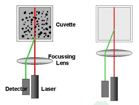
Measurement zone moves to reduce multiple scattering and collective diffusion
