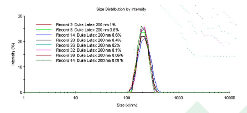
Latex 200nm measured with NIBS and <u>on the side of cuvette</u>. With increasing concentration, result remains unchanged
