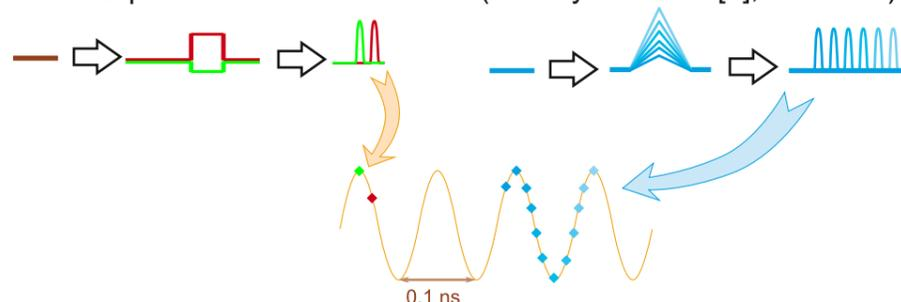
Single XAFS measurements performed on a single period of a microwave (10 GHz) can be produced in the time range of a microwave period (100 ps at 10 GHz). This tool provides a temporal mapping of the surrounding species and resolves the influence of the electro-magnetic field on their interaction.
