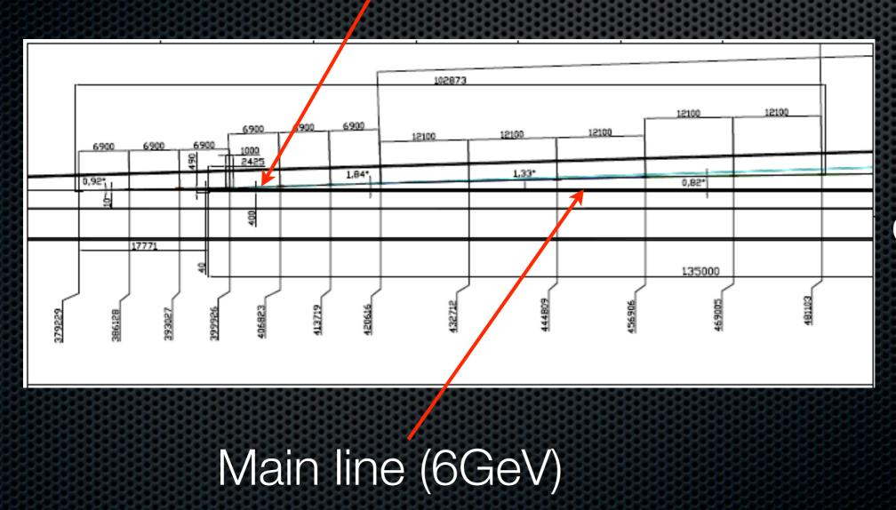
Separation of the beamlines at the experimental stations must be around 6-7 m
