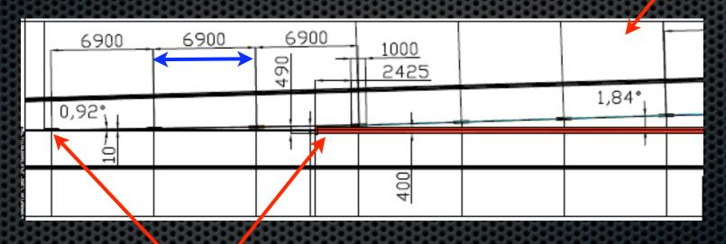
Minimum deflection angle this is due to the accelerating structure for the main line which comes after the switchyard
