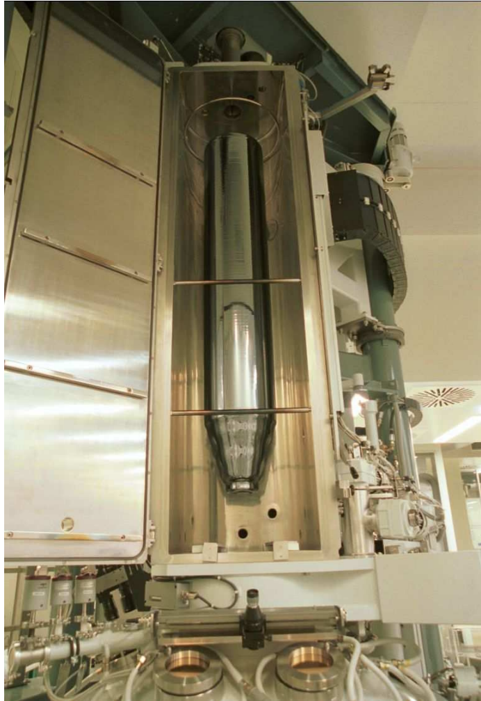
300 mm silicon single crystals grown by Wacker Siltronic AG, weight 250 kg
