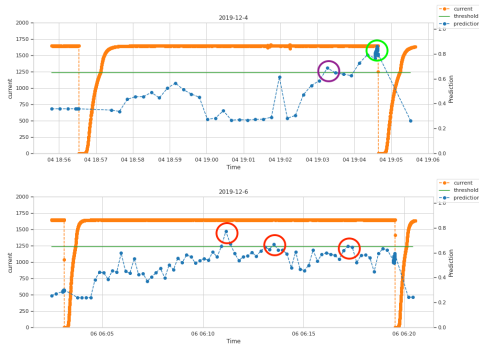
Figure: Screenshots from mimicked live predictions over the validation data. Blue line: prediction value from the model; Orange line: beam current where a drop to zero indicates an interlock; Green line: binary classification threshold.
