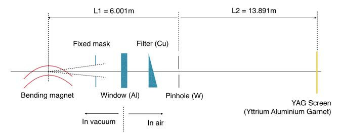
X-ray pinhole camera provides transverse size measurements of the electron beam:
