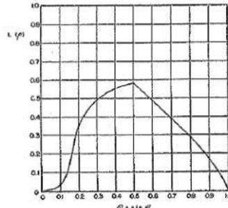
The Bohm and Foldy theory for ion capture shows that the capture efficiency will decrease for decreasing values of  $\sin \phi_s$  below 0.5. However, this calculation does not consider the possibility of modifying the value of  $dF/dt$  while keeping the rotation frequency of the rotco constant
