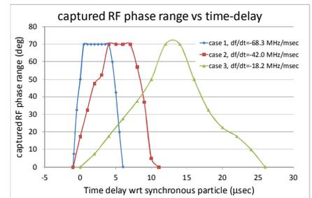
Capture efficiency is considered as the integral of captured RF phase range as function of the width of the time window during which particles are accepted. Case 3 having the smallest rate of frequency change  $dF/dt$  will be the most efficient despite the fact that the width of the RF-frequency window is the smallest for this case.
