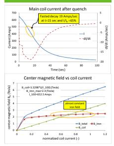
□Obtained from ASG quench model=> After a quench detection a safety circuit to a dump resistor is activated
