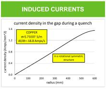
□ Induced magnetic field can be estimated by assuming all currents to be concentrated in a thin sheet. => they are very small (about 40 Gauss)
