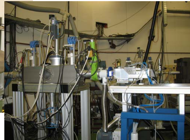
High power solid target With automatic transfer
