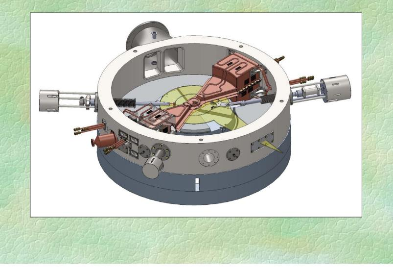
The extraction system of the cyclotron is based on a stripping foil made of carbon in which H<sup>-</sup> ions are converted into protons.
