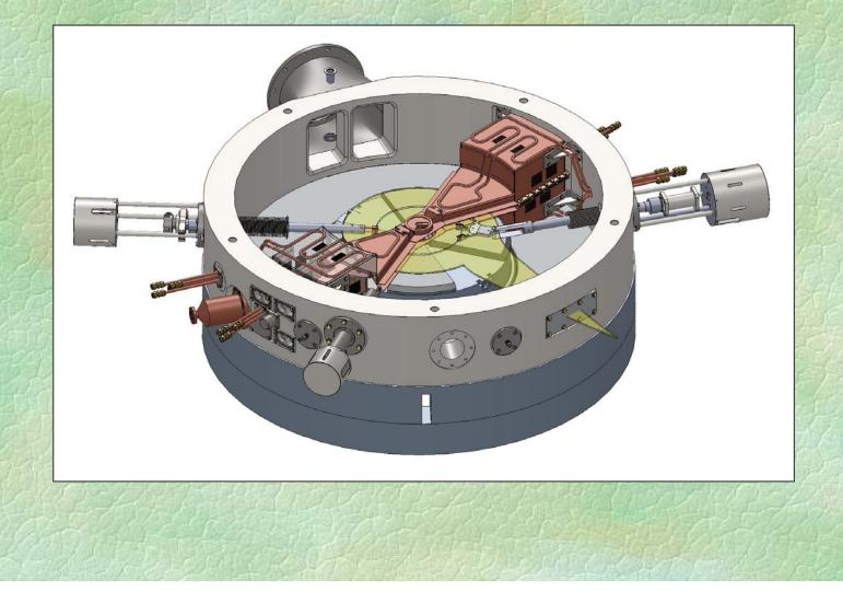
The RF system of the cyclotron includes two  $\lambda/4$ -resonators placed in the vacuum chamber – between the electromagnet valleys.
