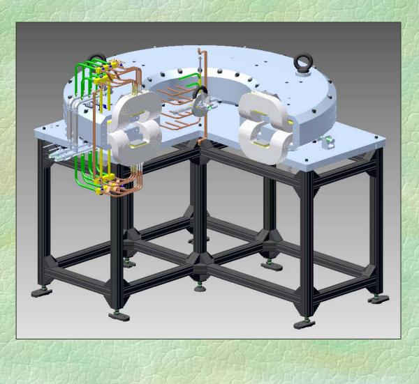
The switching magnet can bend the beam for  $\pm 15^{\circ}$ . It enables one to connect to the complex three experimental channels. The transport and preparation system also includes two diagnostic boxes, placed before and after the monochromator, each of them containing a beam profile monitor and a Faraday cup.
