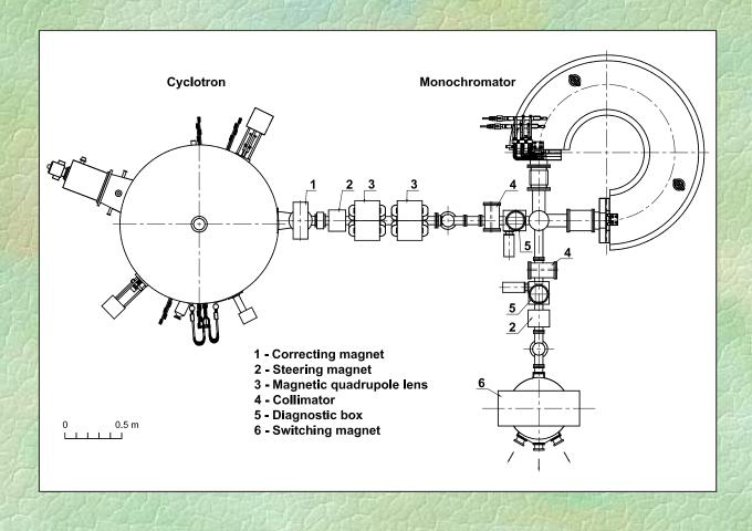
The correcting and steering magnets are used to correct the direction of the proton beam after the extraction from the cyclotron and along the system, the quadrupole lenses are employed to focus the beam at the entrance of the monochromator, the monochromator is used to define the energy and reduce the energy spread of the beam, and the switching magnet is employed to direct the beam toward the target to be analyzed.
