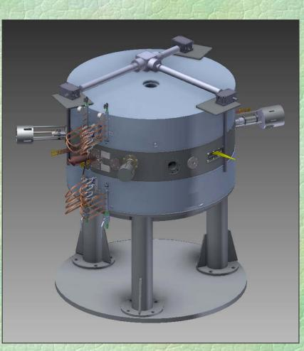
The vacuum chamber of the cyclotron consists of a cyindrycal body and the upper and lower plates, which are made of the ferromagnetic material and belong to the magnetic circuit. Each plate is reinforced with an annular extension made of stainless steel.
