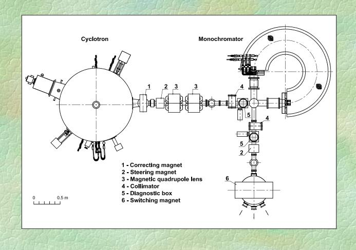
The radius of the monochromator is 600 mm, its effective bending angle is 270°, and it has the variable collimators of the widths of 0.5-2 mm at its entrance and exit.
