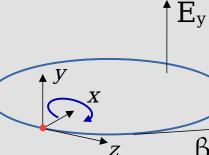
If a longitudinal E-field component is present it will couple to the anomalous magnetic moment and result in a precession in the vertical plane mimicking an EDM.
