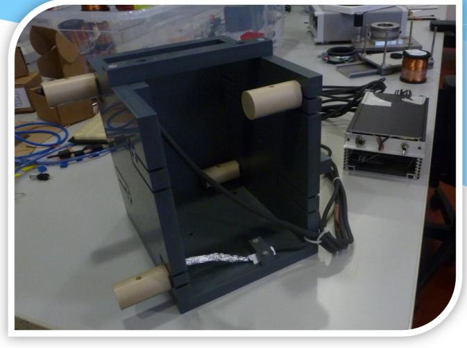
Measurement of external magnetic fields and all gradients with frequency up to 1kHz
