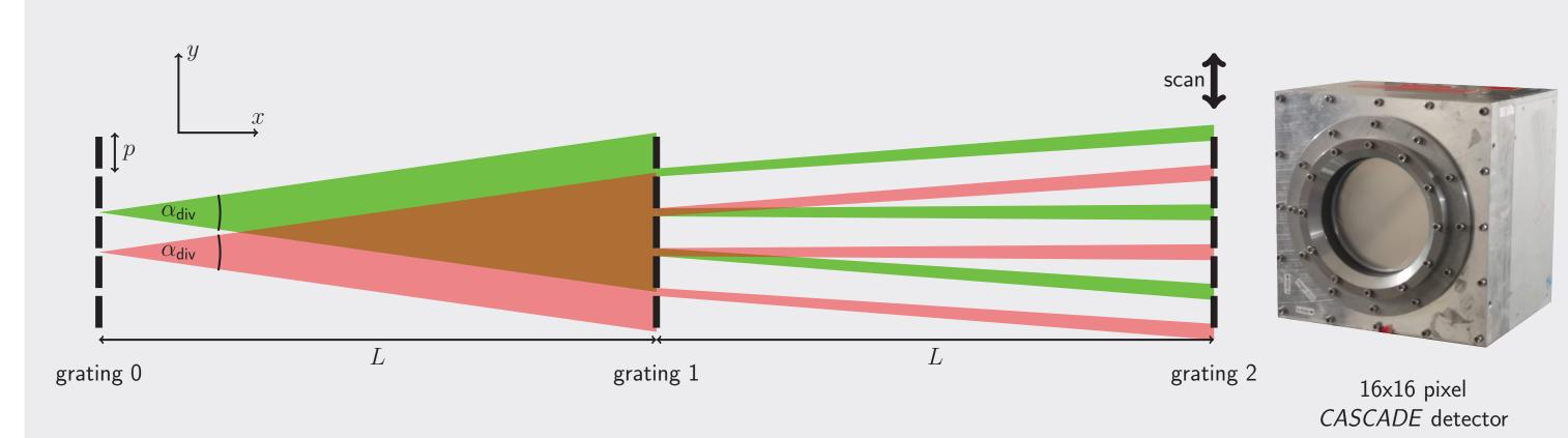
► Transverse scan of grating 2 Oscillating intensity pattern • Visibility:  $\eta = \frac{N_{\text{max}} - N_{\text{min}}}{N_{\text{max}} + N_{\text{min}}}$
