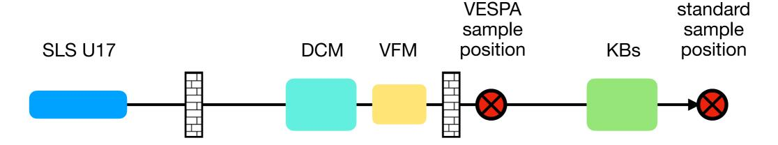
Flexible endstation at PXI 2<sup>nd</sup> source to accommodate different types of serial crystallography experiments and sample delivery systems.
