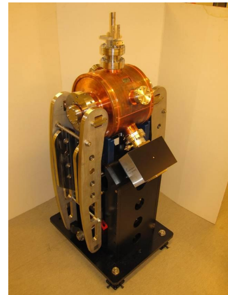
Harmonic Cavity in operation at MAX IV
