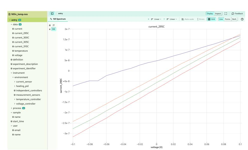
**Generic visualization tool** *h5web* provides plots automatically according to the specification in the data model. Temperature-dependent IV-curve measurements are plotted with different colors.
