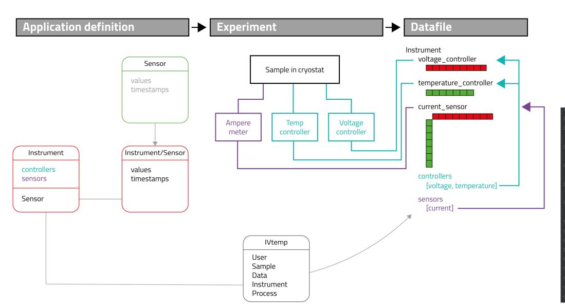
Reuse of Sensor\_Scan modeling arbitrary scan axes under Instrument. The fields independent controllers and measurement sensors refer to sensors acting as scanning axes or measured values.
