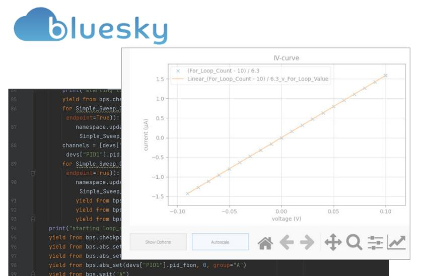
Control and Data Acquisition systems (EPICS / Bluesky [4]) can be configured to store data according to the specified data model. IV\_temp is expressed in NeXus as NXiv\_temp allowing standardized data stored in hdf5.
