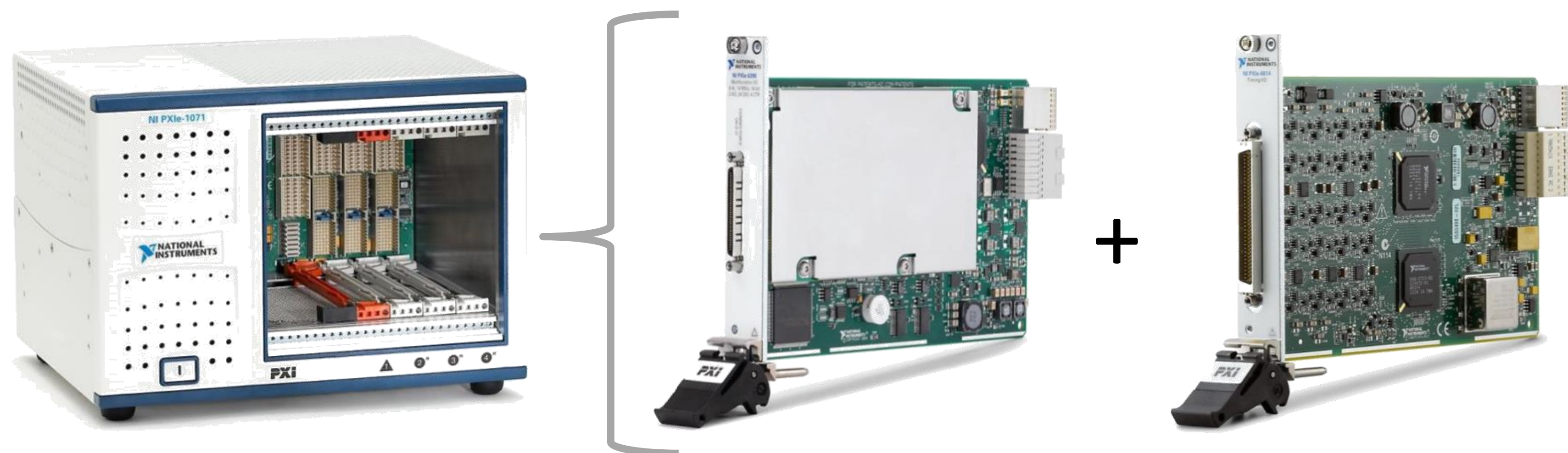
Figure 2. The Debye DAQ hardware is based on the National Instruments PXIe line. The PXIe-6396 3 multifunction I/O module 18 bit analog input sampling at 14 MS/s on up to 8 channels, while the PXIe-6614 4 counter/timer module provides quadrature encoder position sampling. The system is configured to sample based on a common clock generated by the backplane, and ensures both long term hardware-level synchronization of data acquisition and simultaneous triggering of data acquisition.
