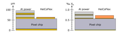
Note 1: Drawn to illustrate total stack thickness. The HeiCoFlex would be on the bottom, of course. Note 2: No need for impedance controlled Al layers allow to drop some polyimide. Hence thinner than LTU.  $M_3$
