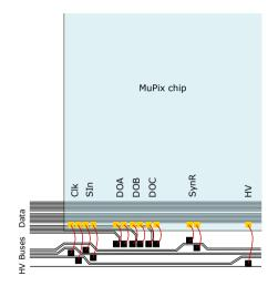
Sketch of a possible routing and bonding scheme.
