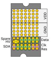
The pad arrangement on the interposer must follow an optimised pattern for this technology:
