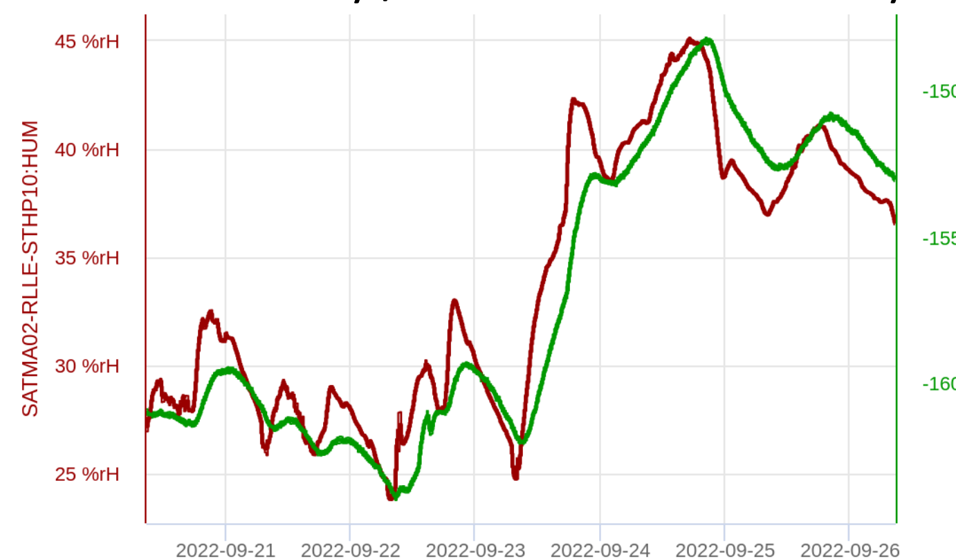
Figure 5: Phase drift vs. humidity
