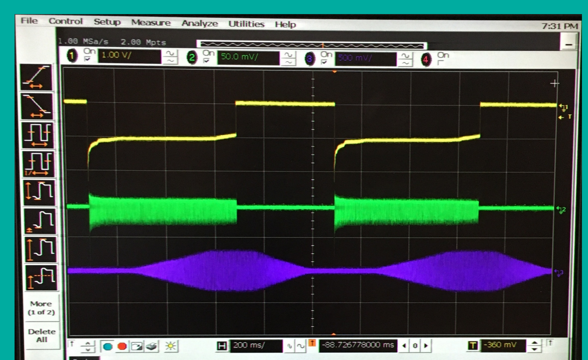
Booster injection. Yellow: Parametric Current Transformer; Green: Fast Current Transformer; Lilac: RF envelope.
