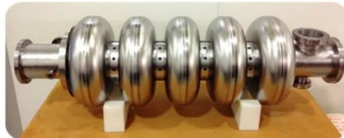
Figure 1: High beta 704.42 MHz undressed cavity.
