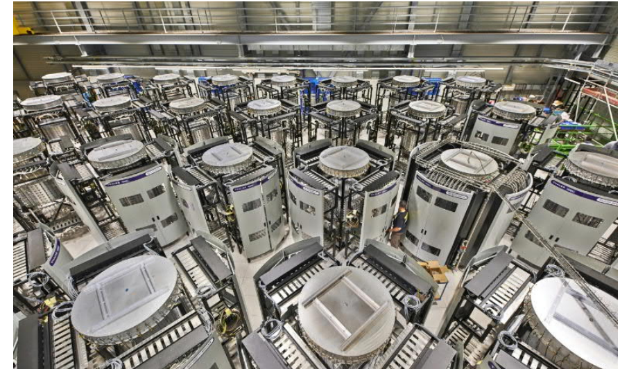
Fig3 – SPS Solid-state amplifier systems (32 towers of 140kW!)
