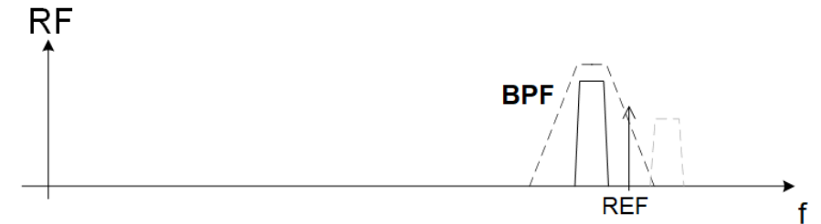
Fig17 – 200MHz Cavity-Controller vector modulator spectrum
