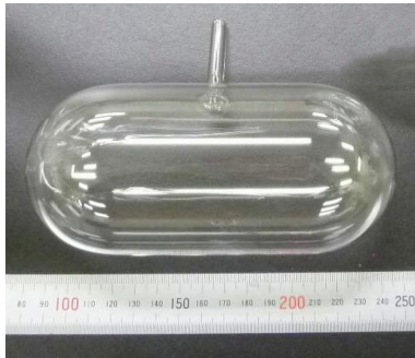
Prototype Gas Cell \varnothing 74 mm x 152 mm (picture from T. Ino)
