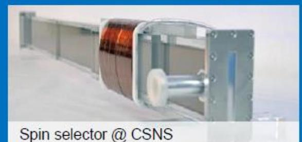
Spin selection: 2V-cavity combined with RF spin flipper
