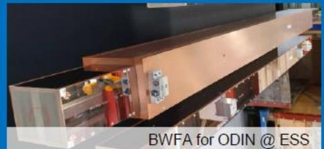
Complex elliptic guides made from glass, Al, or Cu
