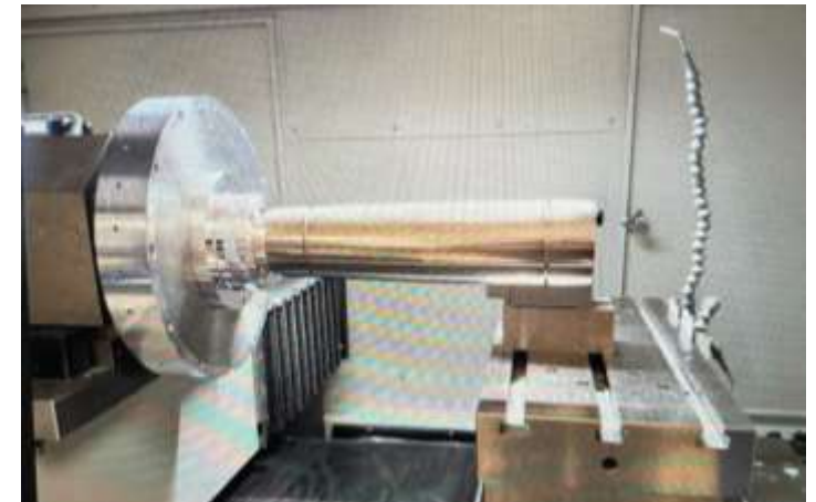
Imaging Mandrel being turned at long last (02 MAR 2023)
