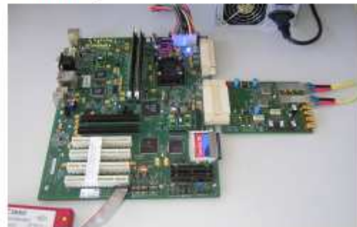
Test setup: ML510 Vertex 5 evaluation Board + XPB personality board
