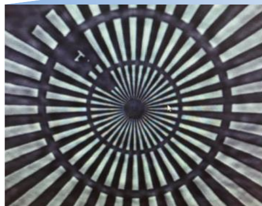
2020: 2D image, Siemens star Resolution \approx 17nm
