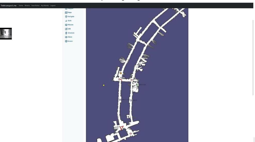
Trajectory planning/2D LIDAR localization stack based on customized algorithms and patched Google Cartographer
