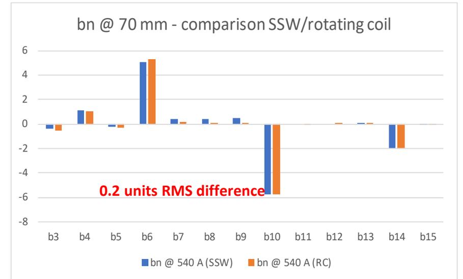
Harmonics fitted to actual flux spanned
