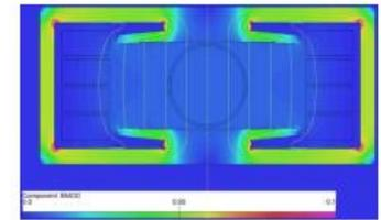
Conceptual design of FCC-ee booster dipole magnet
