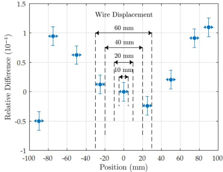
Wire offset  $X_2-X_1$ : trade-off between higher S/N and effect of  $B_3$
