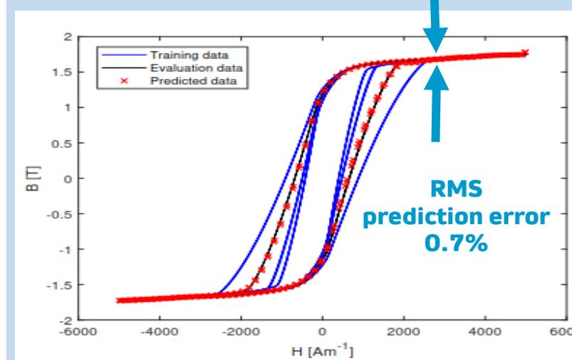
ARMCO ring sample with varying excitation ramp rate
