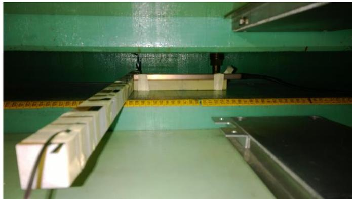
Straight samples tested open-circuit in 1T field
