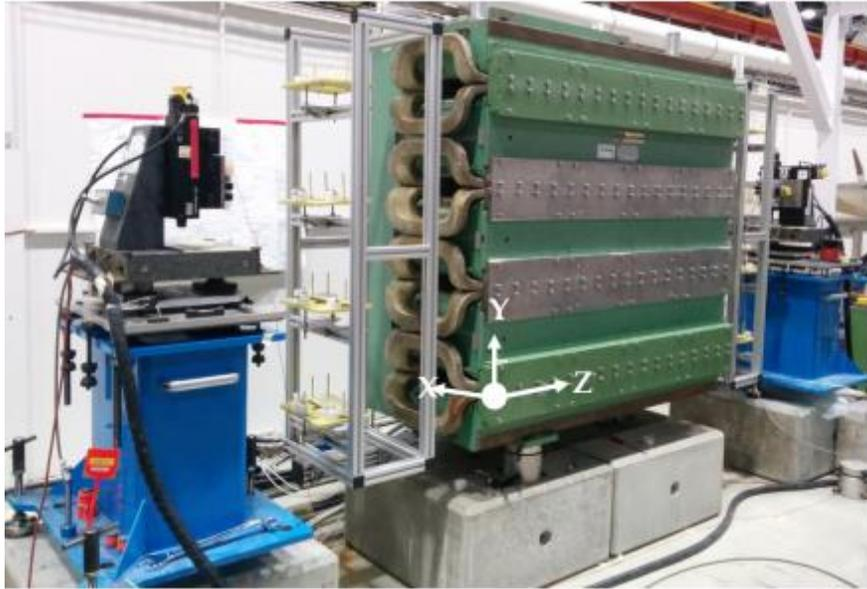
Pulsed-mode flux integration in PS Booster main dipoles
