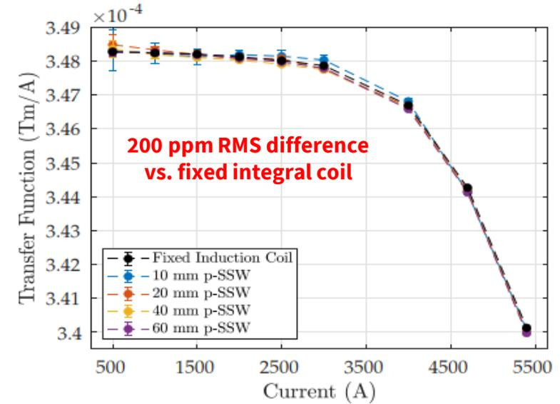
Standard static SSW measurement added in to recover initial level at  $I_0$
