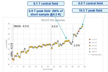
Support to collaborations, e.g., testing at SM18 of PSI CCT Nb<sub>3</sub>Sn dipole magnet model
