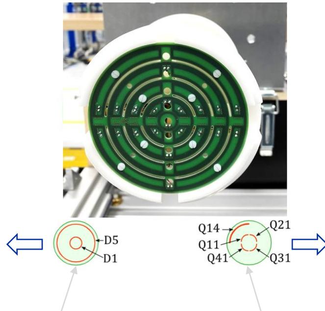
4x360° + 1 central, 6-turn concentric coils for axial and radial field profile
