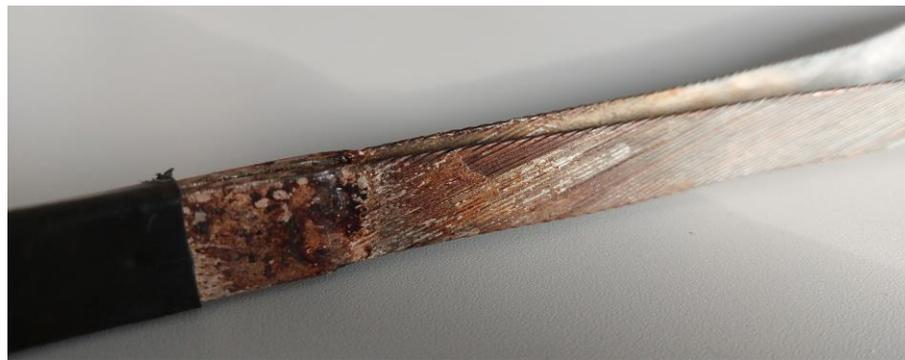
2x 18 kA current leads, to be refurbished with SnAg
