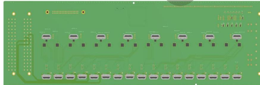
In-house developed **17x8** bidirectional USB matrix switch, freely available on <https://ohwr.org>
