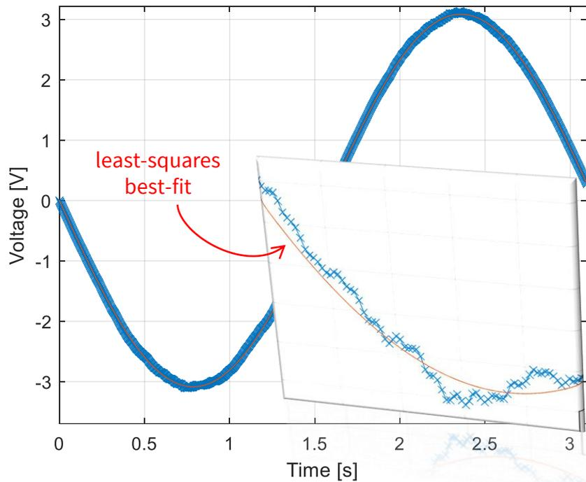
Derive  $\omega(t)$  and then  $\theta(t)$  from the sine wave that best-fits  $V_{\text{coil}}(t)$
