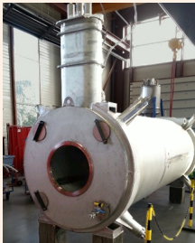
24 TONS, WARM BORE 600MM, 4,25T NBTI LIQUID HELIUM 4,2K 3500 A
