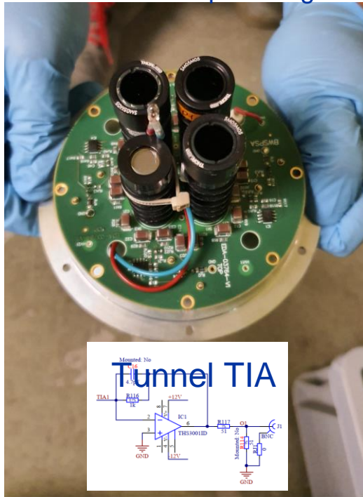
PMT with custom powering base
