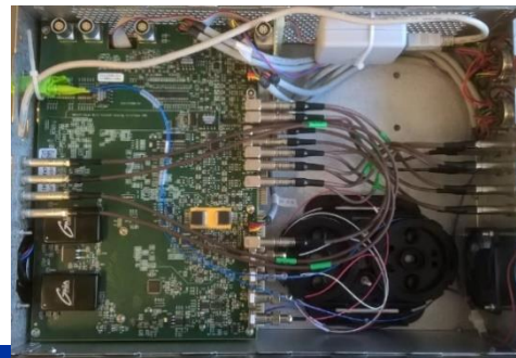
BWSAIF (Motor inverter) bench Python based script using JTAG (soon to be migrated to Ethernet)
