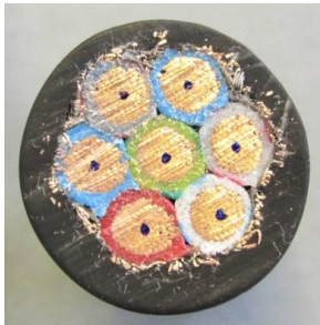
Cross-section “PL7SE” 7 conductors of 6mm 2 with outer shielding. EMC connector mounting procedure EDMS-2172897
