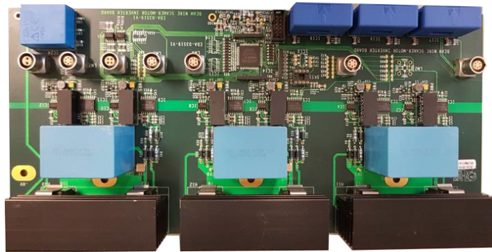
IGBT based Three phase full bridge inverter
