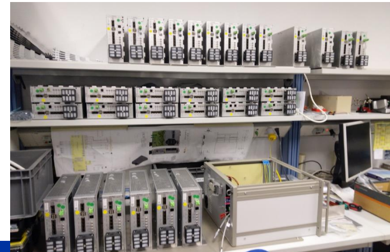
BWSAIF (Motor inverter) bench Python based script using JTAG (soon to be migrated to Ethernet)
