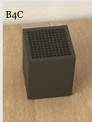
Double collimator – channel size 3 mm x 3 mm
