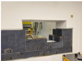
Use of new developed borated mineral cast
