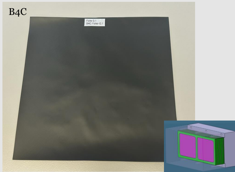
Thin foils – thickness 100 \mu\text{m} (size 200 mm x 200 mm)
