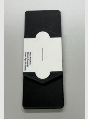
Apertures – opening can be 0.1 mm (slite width)
