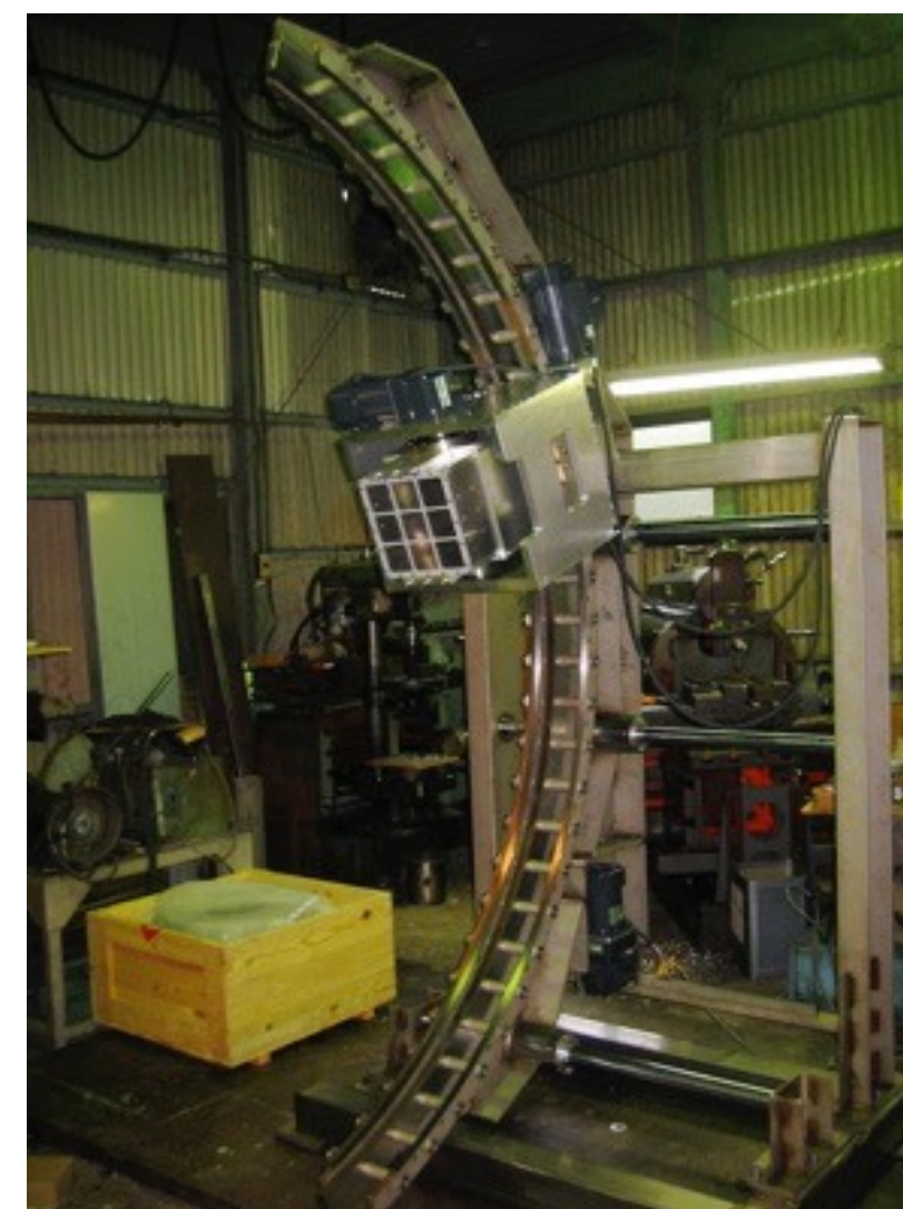
BGO crystal array on a movable stand to tag photon
