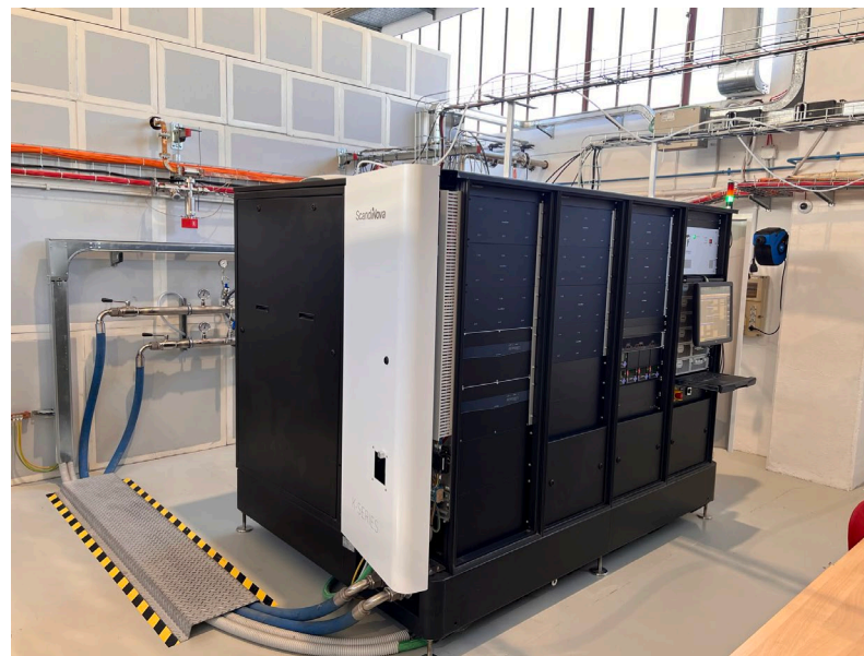
RF Source (Scandinova K400 + CPI klystron VKX-8311A)
