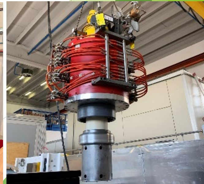
RF Source (Scandinova K400 + CPI klystron VKX-8311A)
