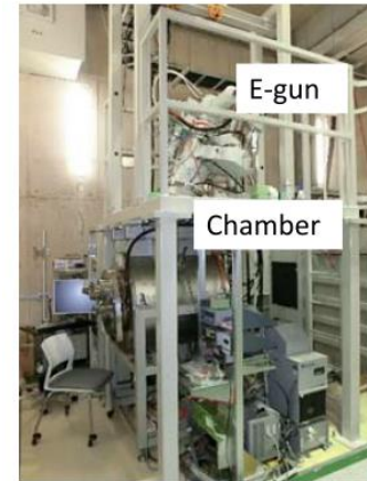
Electron gun: JEBG-3000UB manufactured by JEOL Ltd.
