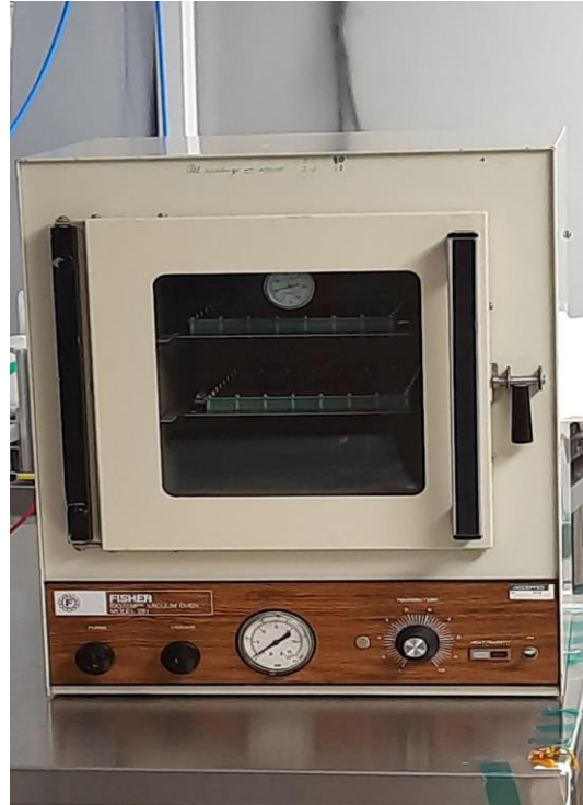
Detectors being baked at 50 degree Celsius
