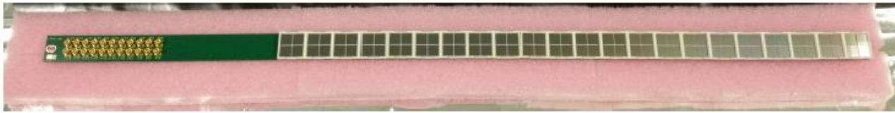
Figure 2.17 PCB used to align the MPPCs.
