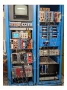
Two beam development shifts partially dedicated to the selector. Setup put together in beamline 1B with scintillation counters & NIM logic.
