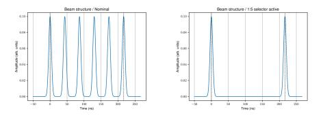
When enabled, the "5:1 selector" suppress 4/5 bunches, bringing the repetition period to  $\approx 215~\text{ns}$
