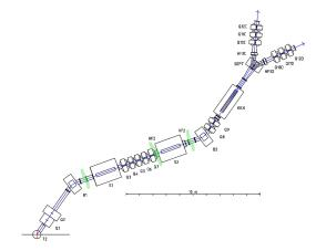
The momentum bite is not precisely known (depends on slits positions). A detailed G4Beamline sim has been developed by TRIUMF's CMMS group.
